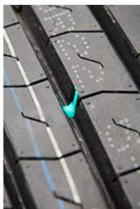
Punctured tyre with Ultra-Seal
